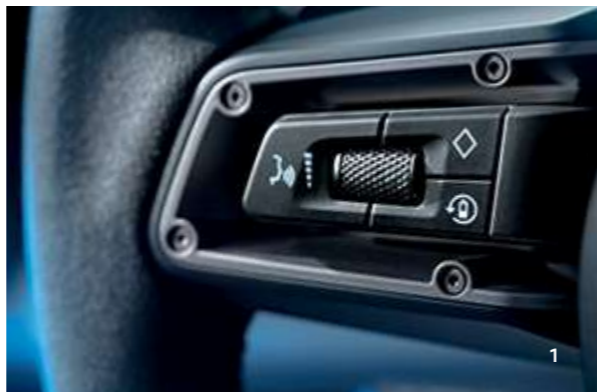
1 Recuperation button on the steering wheel for selecting recuperation stages
